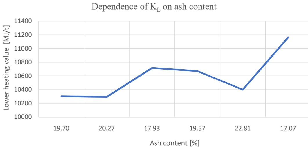
Figure 4. Dependence of  $K_L$  on ash content
