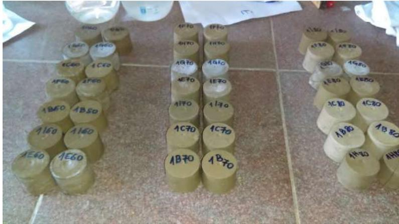
Figure 3. Geopolymer samples that have undergone heat treatment
