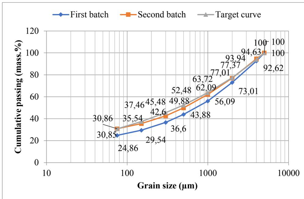
Figure 1. Particle size distribution of mixture in the first and second batch and target particle size distribution
