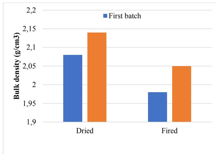
Figure 2. Effect of particle size distribution and thermal treatment on bulk density
