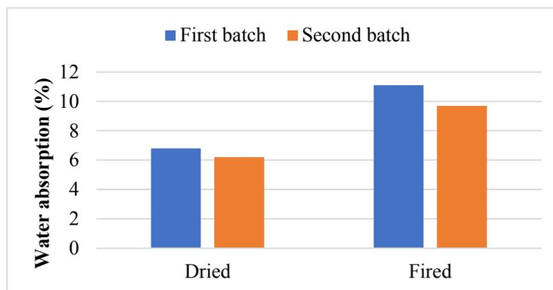
Figure 4. Effect of particle size distribution and thermal treatment on water absorption
