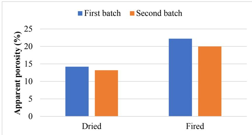
Figure 3. Effect of particle size distribution and thermal treatment on apparent porosity
