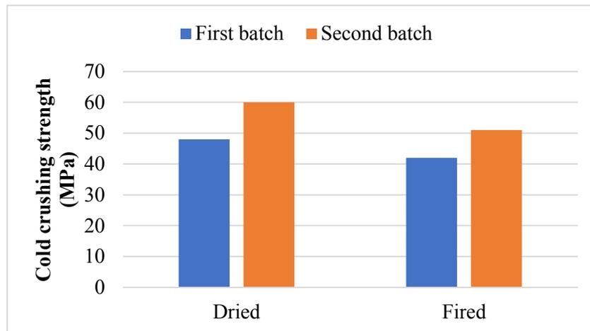
Figure 5. Effect of particle size distribution and thermal treatment on cold crushing strength
