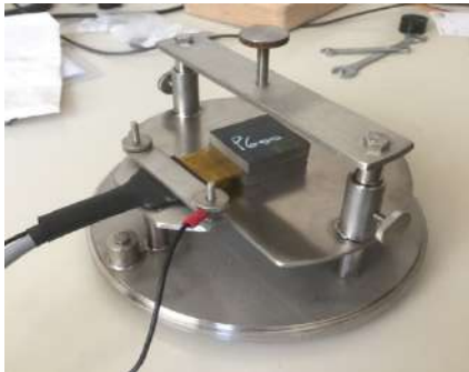
Figure 3. Measuring sensor sandwiched between two halves of a sample during measurement.
