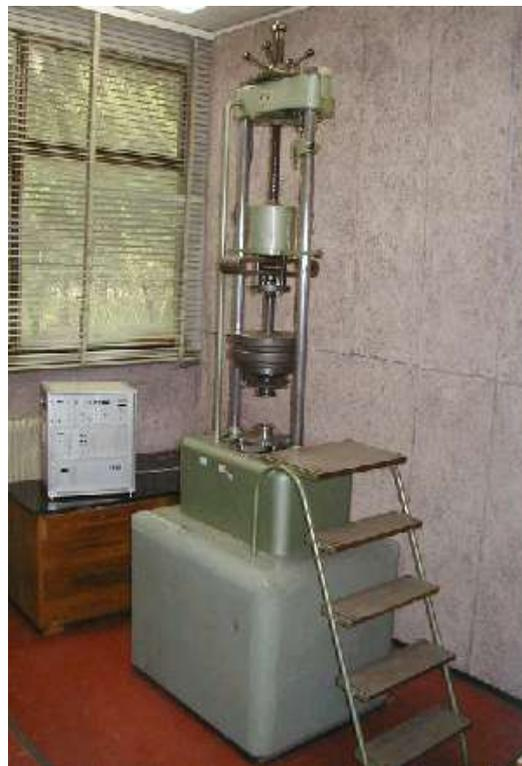
*Figure 2. High-frequency pulsator "Amsler" for dynamic testing [3]*
