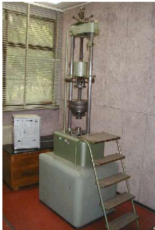
Figure 2. High-frequency pulsator "Amsler" for dynamic testing [3]
