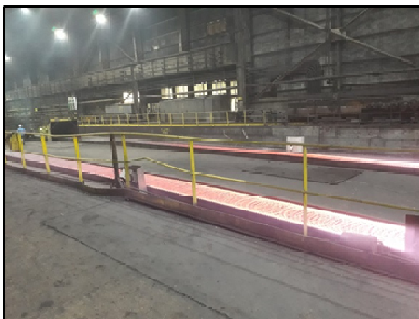
Figure 2.3. Glowing coil at Stelmor conveyor
