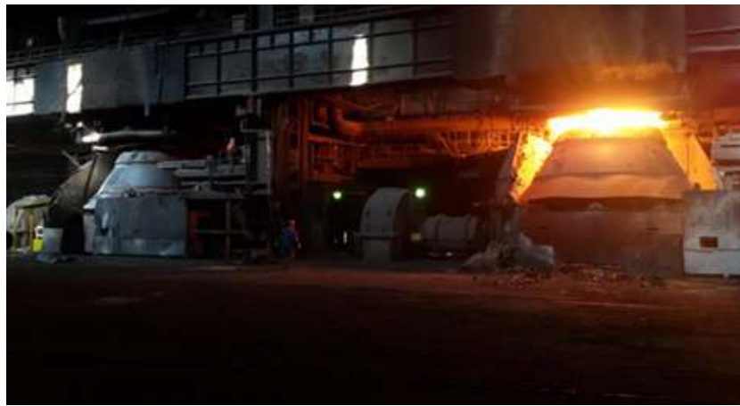
Figure 2.1. Basic oxygen furnace in the company ArcelorMittal Zenica
