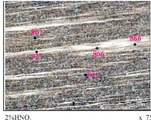
Figure 3. The appearance of the microhardness imprint on the steel sample
