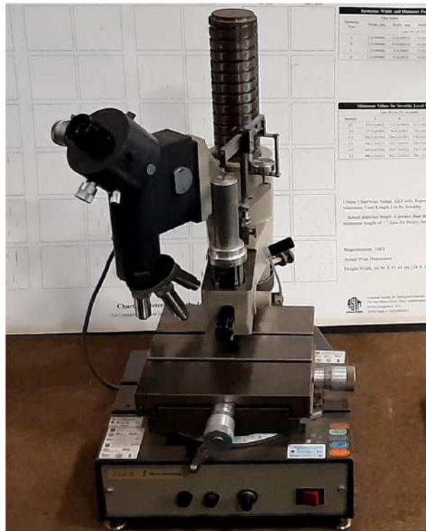
Figure 1. Zwick devices for measuring microhardness testing
