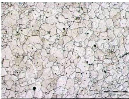
low carbon steel grain size (NITAL)
