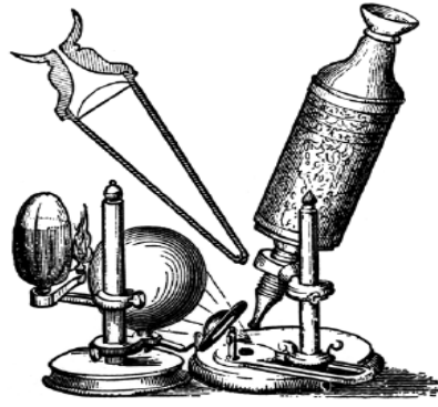
Figure 3. Sketch of the microscope used by Robert Hook, in 1665. [2]
