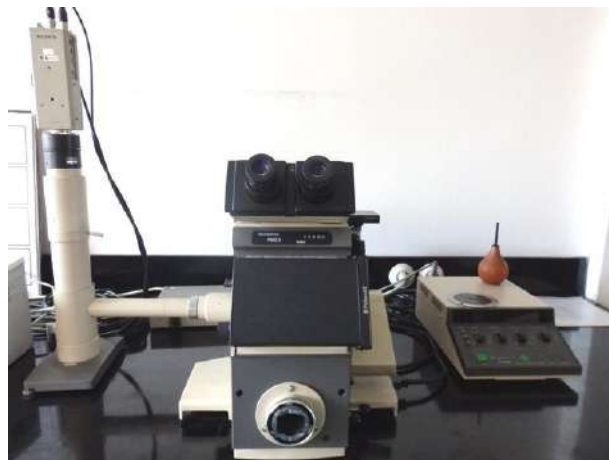
Figure 5. Layout of a modern light optical microscope
