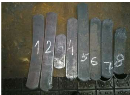
Figure 8. The samples after the rolling process was performed [15]
