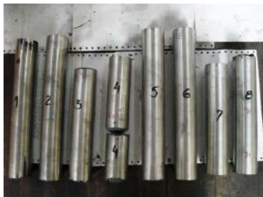
Figure 5. The samples after the completion of forging process and rough machining [15]
