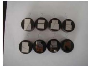
Figure 6. Forged samples for metallographic tests [15]
