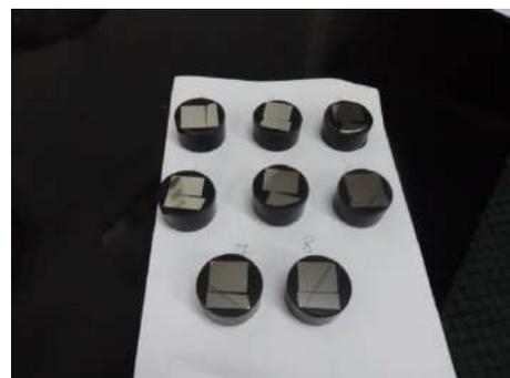
Figure 9. Rolled samples for metallographic tests [15]
