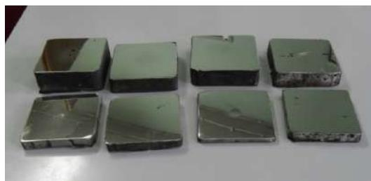
Figure 3. Casted samples for metallographic tests [15]
