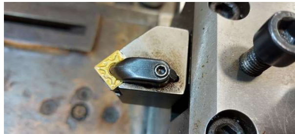
Figure 4. Replaceable cutting insert type SNMG 120408-MAUS735
