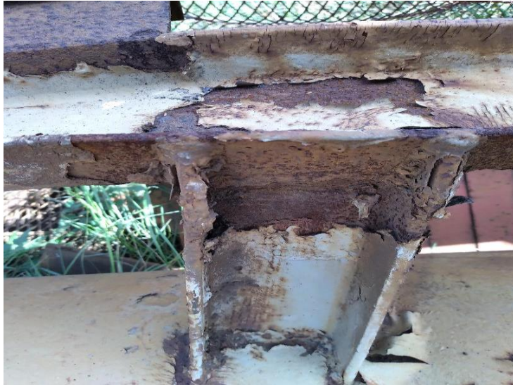
Figure 6. Detailed position of a deeply corroded section of a broken portal crane
