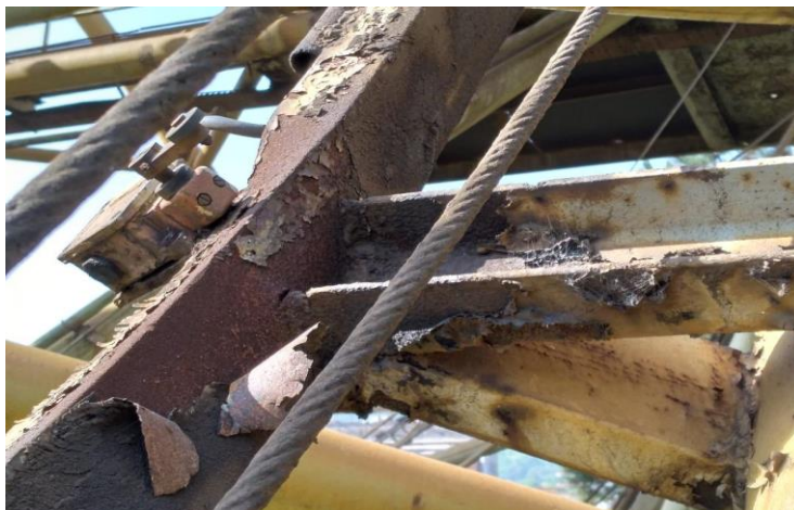
Figure 7. Detailed position of a welded and deeply corroded section of a broken portal crane
