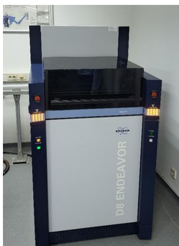
Figure 2. Bruker D8 Endeavor XRD device
