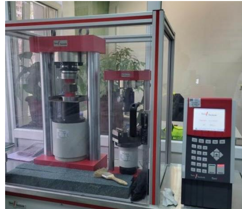
Figure 4. Press for testing compressive and flexural strength
