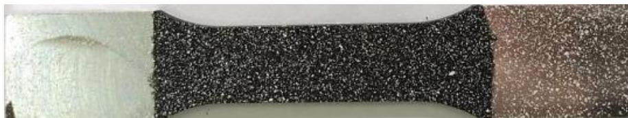
*Figure 2. Dog-bone specimen prepared for simultaneous tensile strength – DIC - thermography testing*
