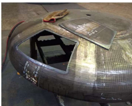
Figure 3. Taking samples from the manufactured floor
