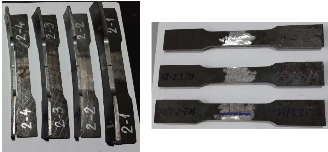
Figure 6. Test tubes for the determination of tensile properties - series II
