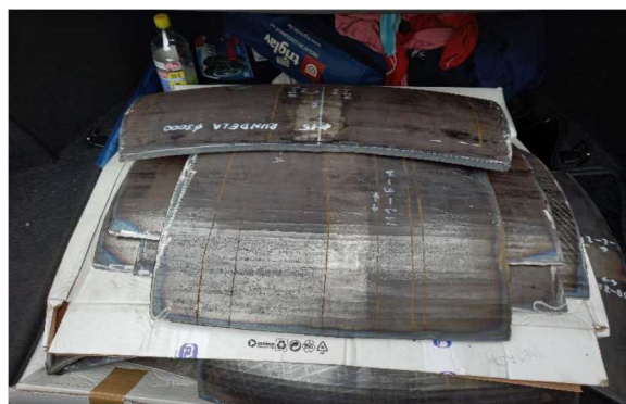
Figure 3. Taking samples from the manufactured floor
