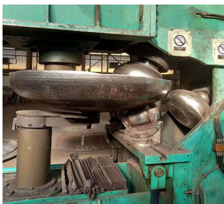
Figure 1. Production of floors by incremental deformation process [2]
