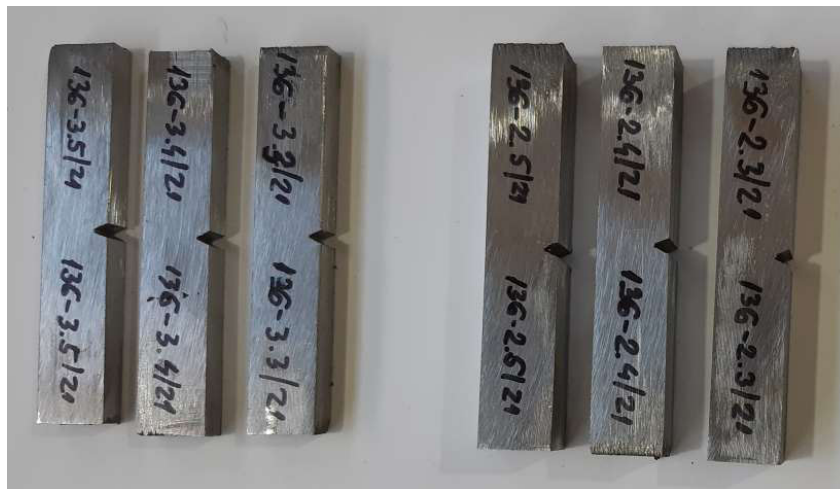
Figure 9. Shape and dimensions of a standard test tube with a V notch for testing by the Charpie method
