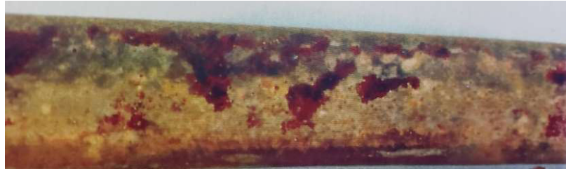
Figure 1. Pipe of steam reheater, after exploitation [8]
