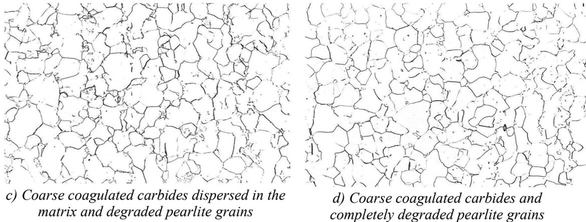
Figure 2. Degradation process microstructure of 15Mo3 steel
