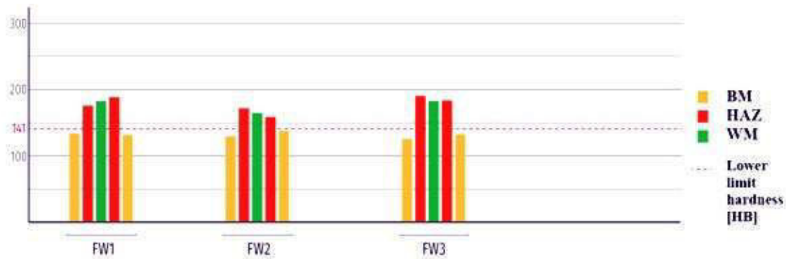
Figure 6. Scattering of hardness on the welded joints of the inlet header of the reheater MPr2
