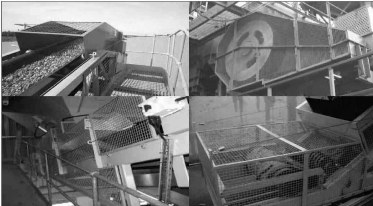
Figure 5. Protection of all rotating and other hazardous parts in technical stone production and processing plants
