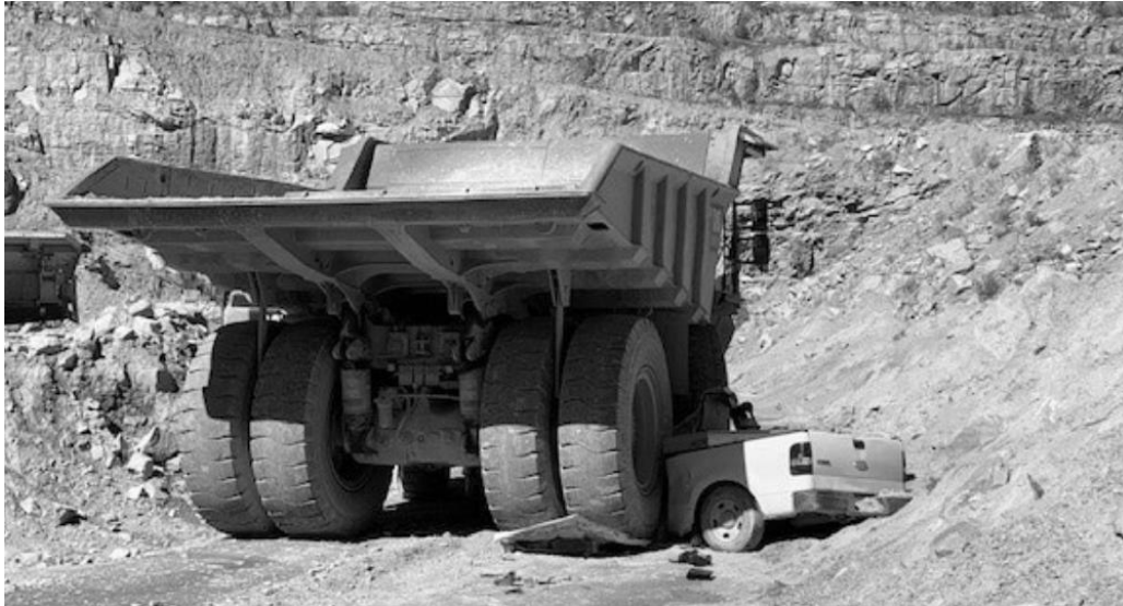
Figure 3. Collision of a dumper and a passenger car in a quarry [17]
