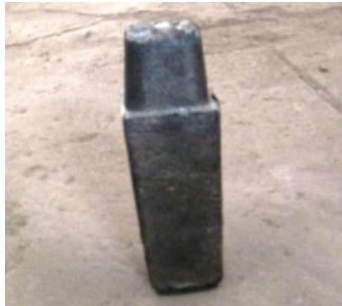
Figure 4. Ingot after the solidification process [5]
