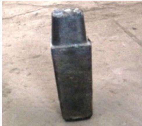
Figure 4. Ingot after the solidification process [5]
