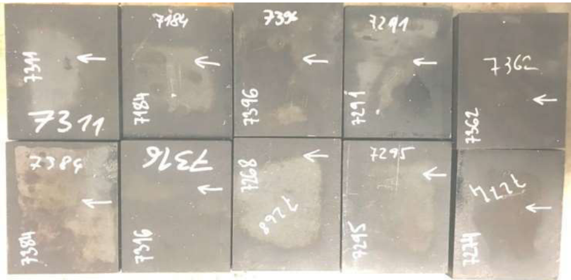
Figure 1. Samples for testing microstructure and grain size taken from melts from T-1 to T-5
