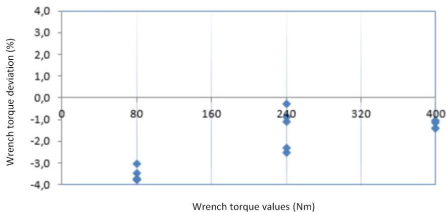
*Figure 2. Graphic representation of torque wrench deviation*
