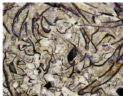
b) etched by nital 2%, magnification 100x
