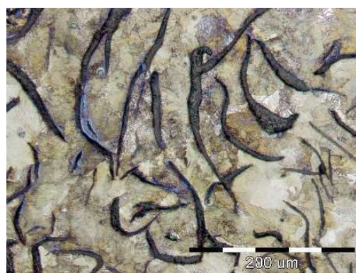
d) etched by nital 2%, magnification 200x
