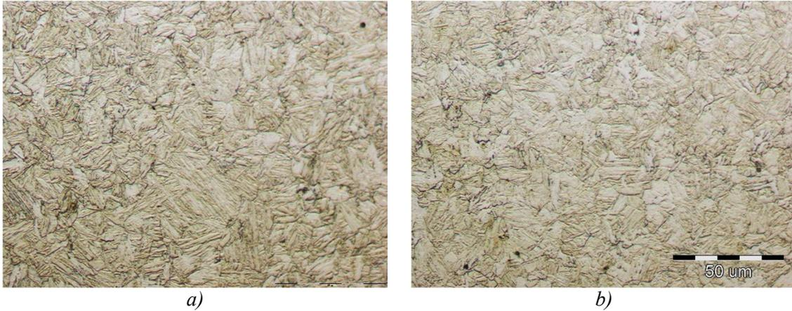
Figure 9. The microstructure of the sample cooled in the oil with a mixing of 750 rpm: a) surface and b) center, x500
