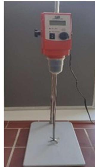
Figure 1. Digital overhead Stirrer LLG-uni STIRRER OH2
