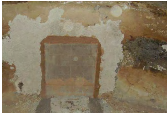
Figure 8. Protection of tundish front side, area of metal impact jet zone with installing of tundish protection plate. [3]
