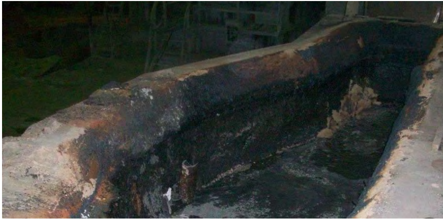
Figure .: Tundish lining based on slurry mix, after lining lifetime.
