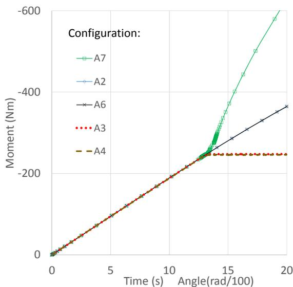
*Figure 4. Reaction moment for different configurations in crack propagation*
