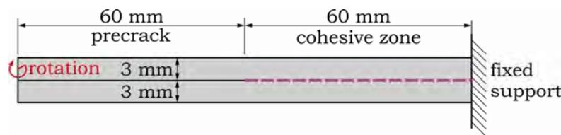
Figure 1. FRMM test configuration.
