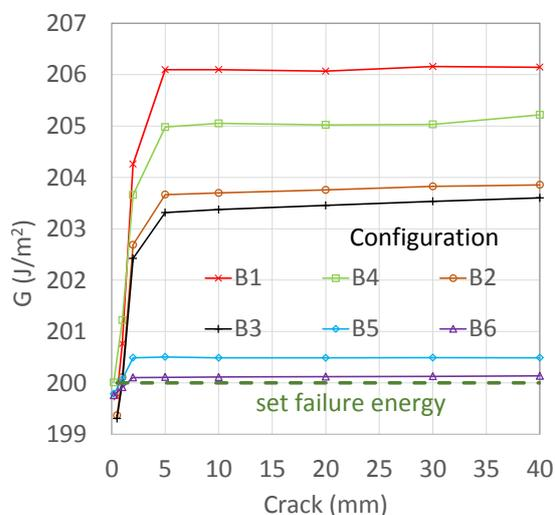
Figure 8. Total energy release rate according to the global approach
