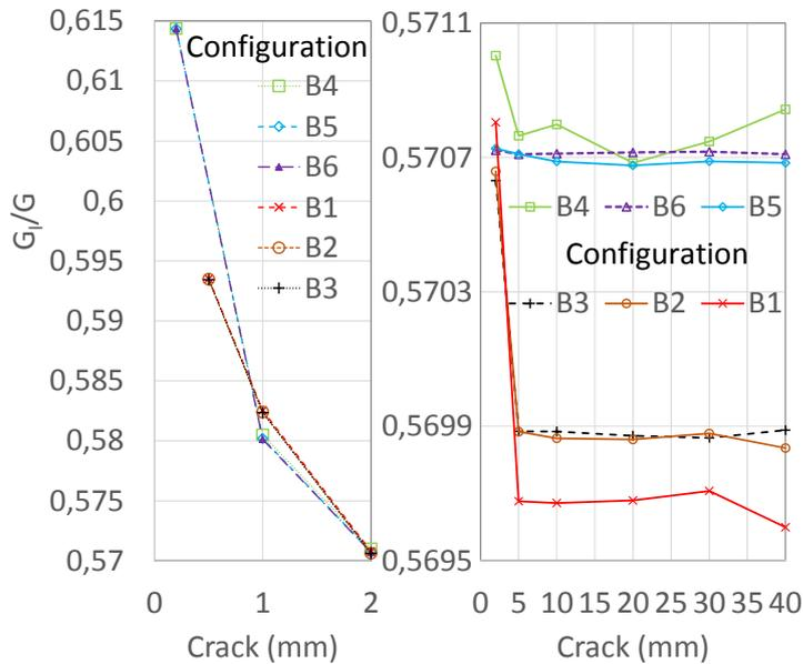
Figure 10. Mode-mixity ratio  $G_I/G$  for different configurations calculated by the global approach
