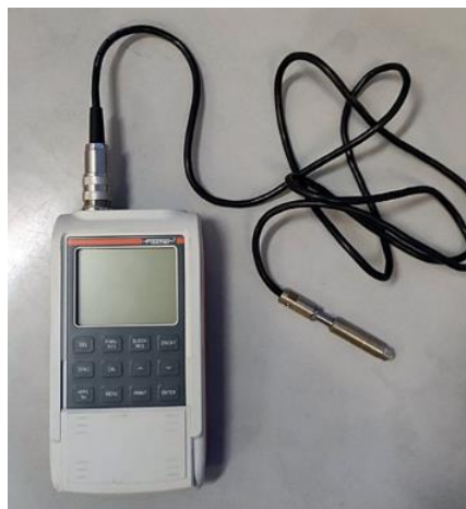
Figure 1. Feritscope MP30E device, manufactured by Helmut Fischer GmbH
