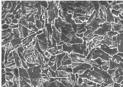
Figure 2. Microstructure of the as delivered steel.
