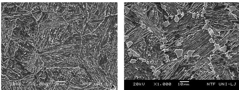
Figure 6. Microstructure after lead bath cooling from 1250 °C (left) and after reheating (right).
