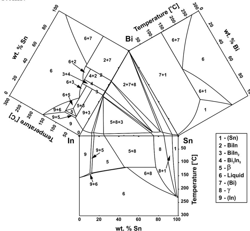
Figure 1. Space ternary phase diagram of Bi-In-Sn ternary system calculated using the thermodynamic parameters from Witusiewicz et al.[15]
