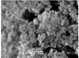
Figure 1. Ultrasil 7005 SEM micrograph [6]
