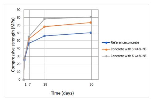
Figure 2. Concrete compressive strength development
