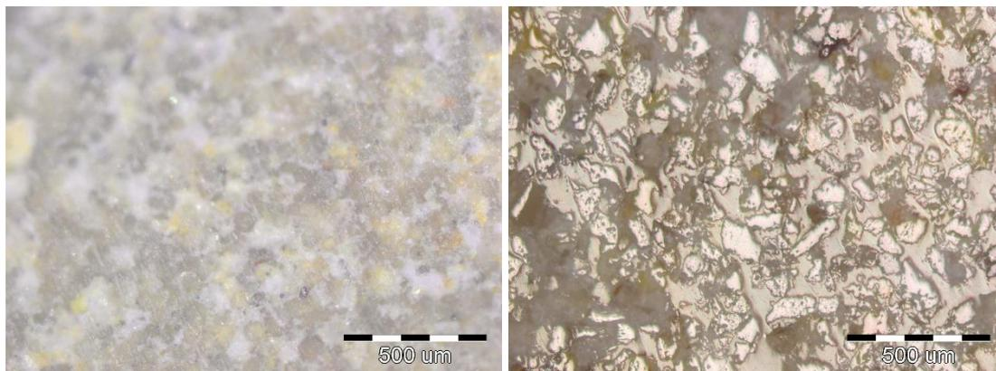
Figure 2. Optical micrographs of the clay (left) and chamotte waste (right)
