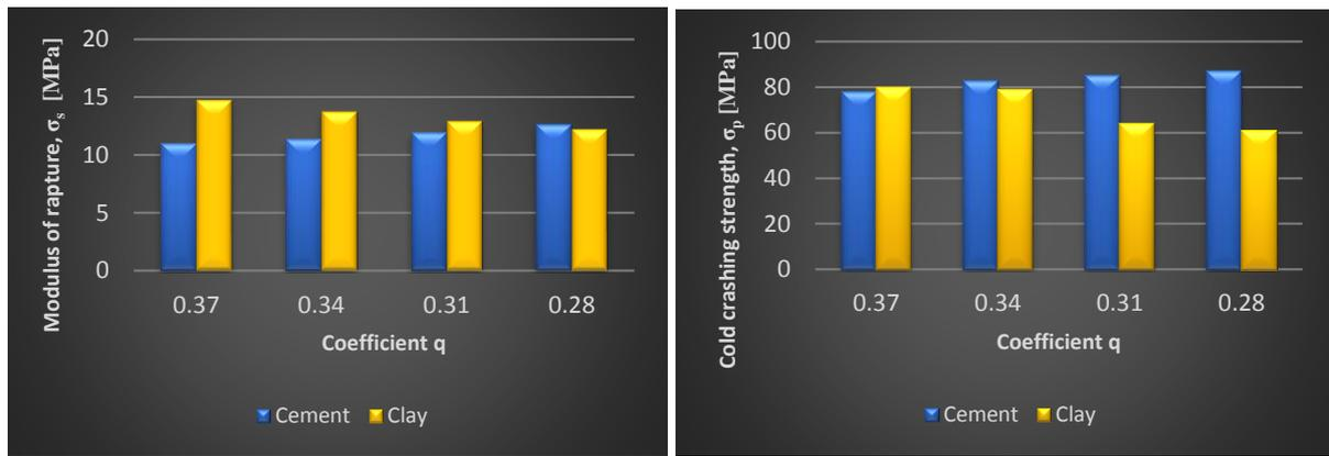
Figure 7. Modulus of rupture and cold crashing strength vs coefficient q
