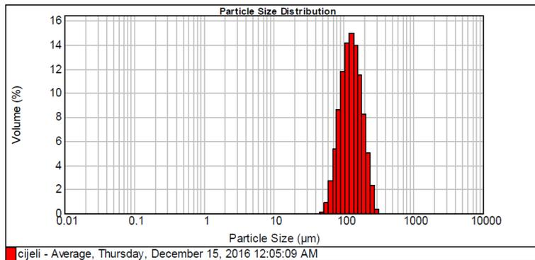
Figure 5. Particle size distribution of chamotte waste fraction 75 – 150 µm
