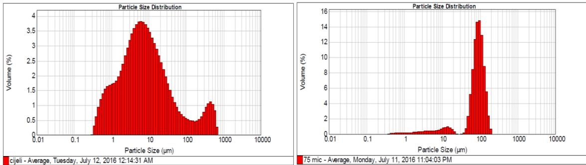
Figure 4. Particle size distribution of clay "Rapajlo": all fractions (left) and fraction 75 – 150 µm (right)
