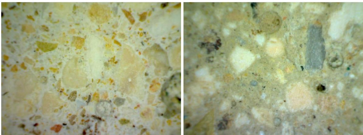
Figure 8. Optical micrographs 60X magnitude of the castable with cement and chamotte (left) and castable with cement, chamotte and clay (right) for q 0.31 by PCE-MM200 Digital Microscope
