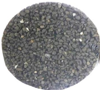
Figure 3. Polished clinker section
