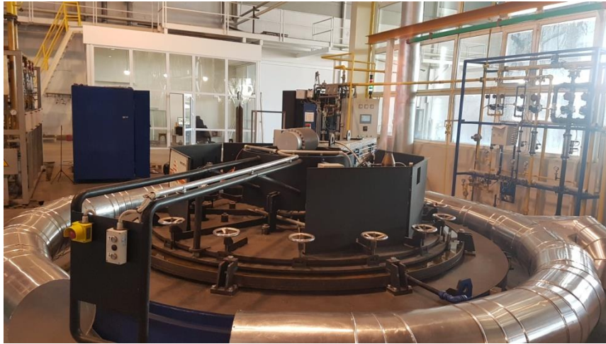
Figure 3. Pit furnace for cementation made by company Bosio
