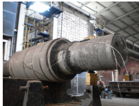
Figure 6. Protection against sagging.
