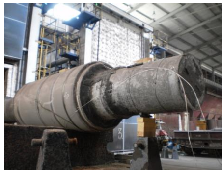
Figure 6. Protection against sagging.
