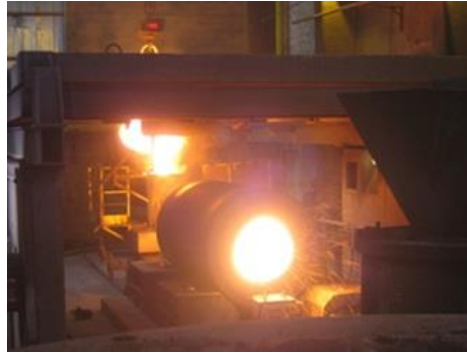
Figure 2. Centrifugal casting of the working shell.
