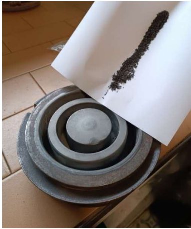
Figure 6. Milling of hydrated TiAl6Nb7 titanium alloy
