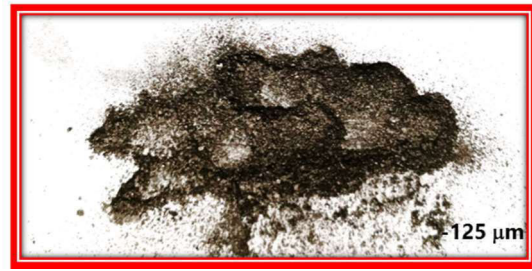
Figure 7. Titanium powder after hydrogenation and milling of TiAl6Nb7 titanium alloy
