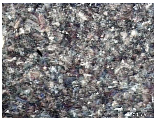
a) carburized surface martensite and retained austenite
