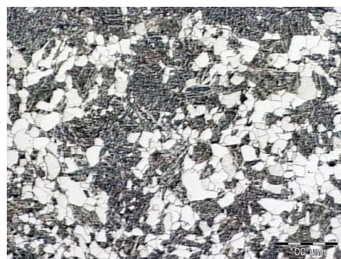
b) core of sample proeutectoid ferrite, pearlite, low carbon martensite
