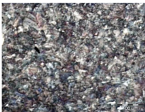
a) carburized surface martensite and retained austenite
