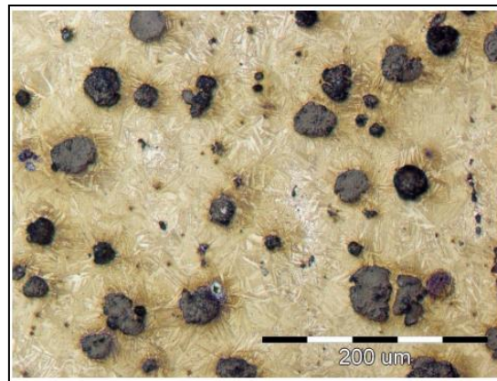
Figure 7. Microstructure of the Ductile iron samples after austempering, 100x
