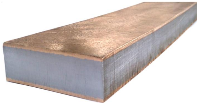
Figure 1. Sample of steel (DC04) strip with CuZn10 clad layers on both contact sides
