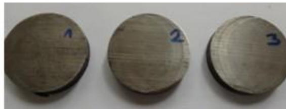
Figure 3. Test pieces for blue fracture testing
