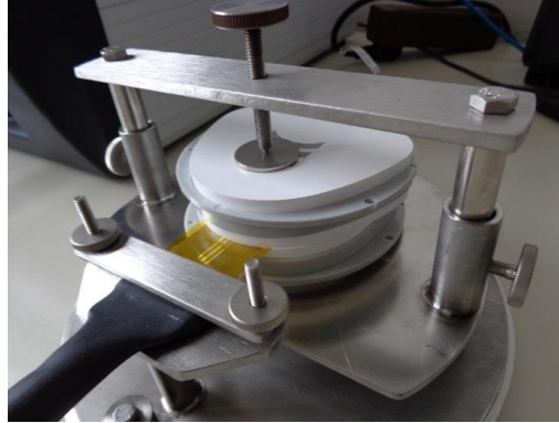
Figure 2. Sensor (Kapton) sandwiched between two halves of a sample during measurement
