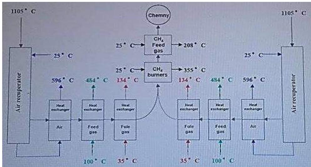
Fig. 19. Heat and energy recovery
