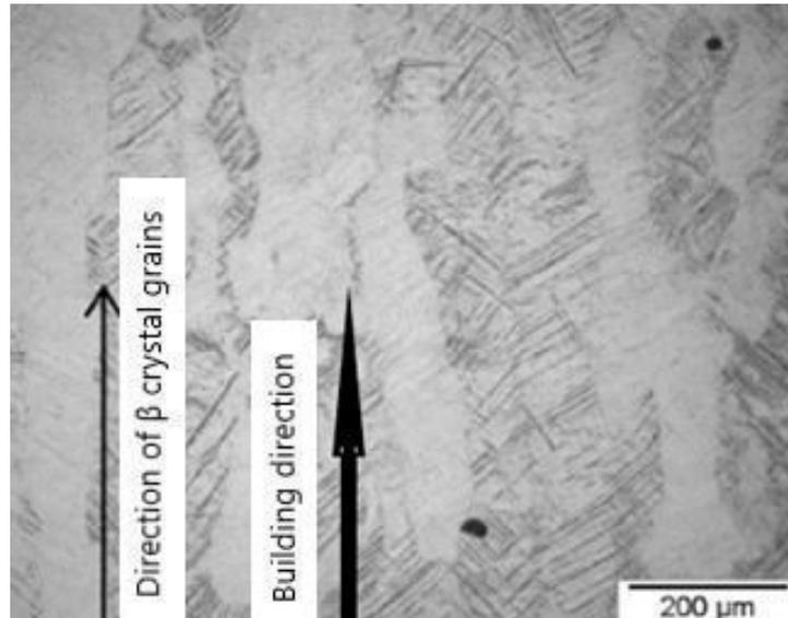
Figure 3. Typical microstructure in SLM manufactured Ti6Al4V sample [12]
