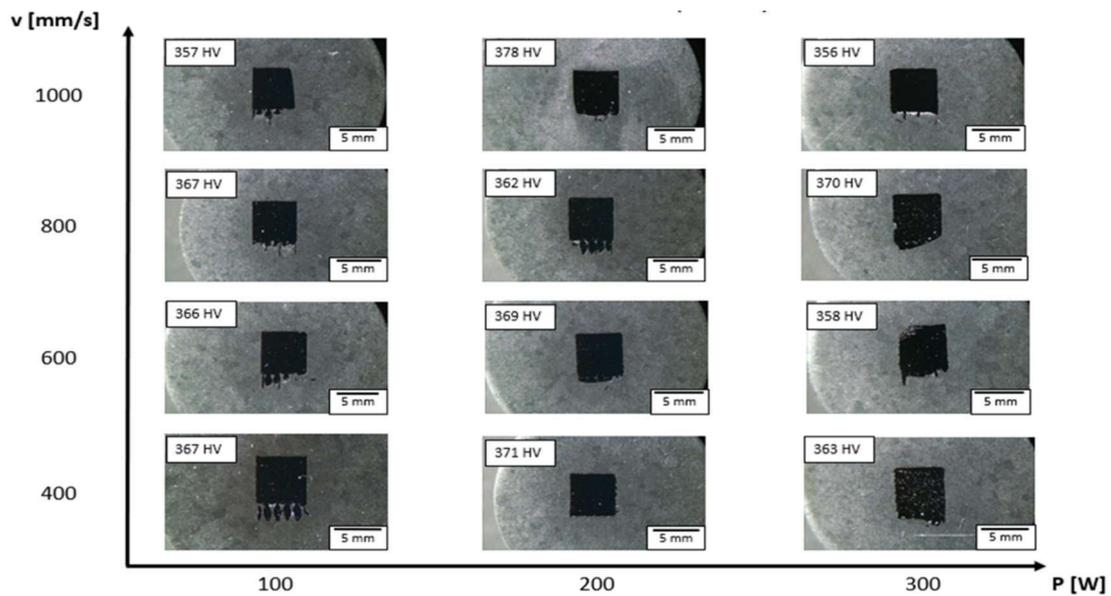
Figure 6. Hardness values at different parameters [HV]
