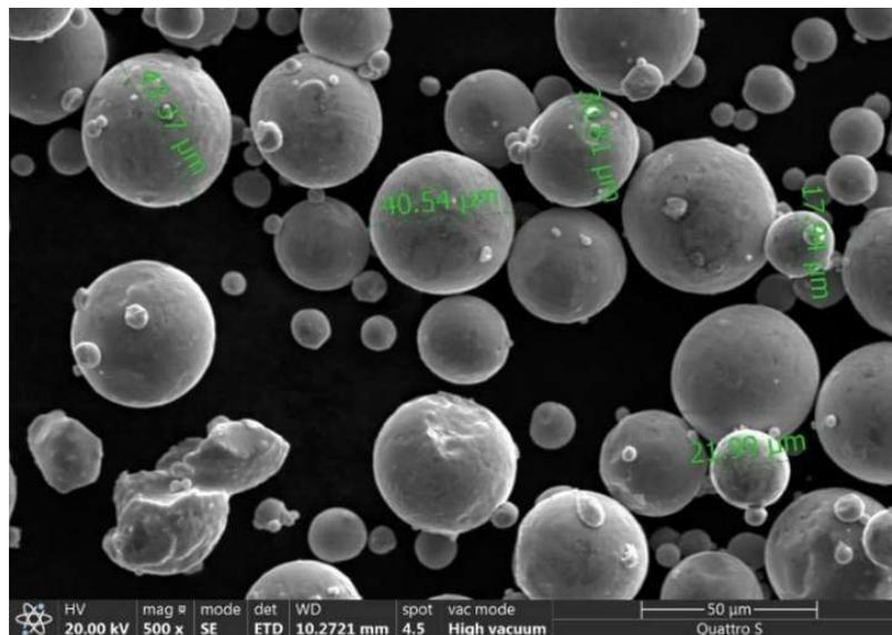
Figure 4: SEM photo of the used Ti6Al4V powder
