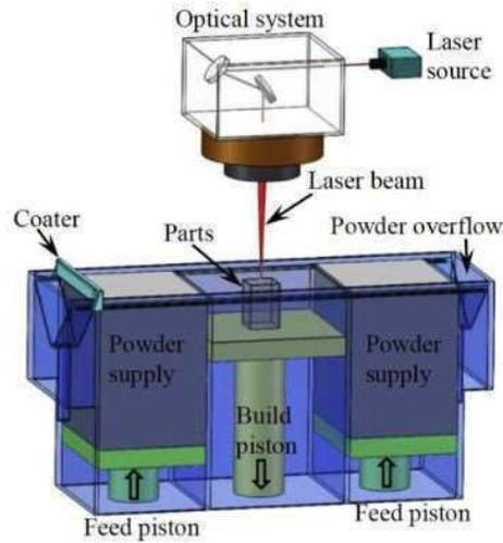
Figure 1. SLM method. Copyright 2019 by Elsevier [5]
